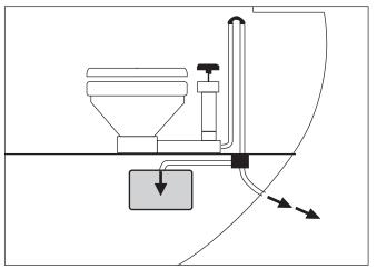
Discharge waste through a Y-valve directly into a non-restricted area, or to a holding tank when within the three-mile limit, using the toilet's own pump and an anti-siphon loop.
