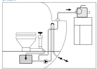
A combination of Options 2 and 3 to give you the flexibility of discharging waste wherever most convenient and without risk to the environment.
