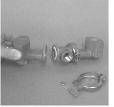
Step 8 Inspect o-rings for wear or damage and replace if necessary.
