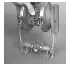
**Step 4** Remove the top manifold and lift the center section off the inlet manifold.
