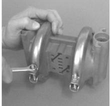
Step 9 Use a 7/16" wrench to remove one set of clamp bands that secure one liquid chamber to the one-piece center section.
