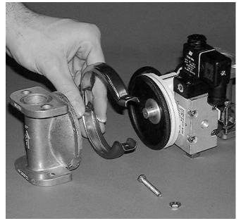
Step 7 After clamp bands are removed, pull chambers away from center section.
