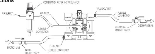
Accu-Flo™ pumps: Accu-Flo™ pumps function with solenoid valves and require an electrical control circuit to supply pulses. Under normal operating conditions, the control circuit is sufficient for starting and stopping the pump. However, the shut off valve (user supplied) installed in the air supply line can be used to stop the pump if necessary. Therefore, it should be located far enough away from the pumping equipment such that it can be reached safely in an emergency situation.
